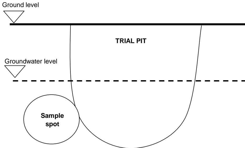
The idea of sample taking is not to take the sample from bottom of the trial pit, because then the sample usually contains extra water and therefore the sample is not representative. Avoiding of surplus water in soil sampling it is advisable that particular soil samples are taken alongside of the trial pit, see below figure.
