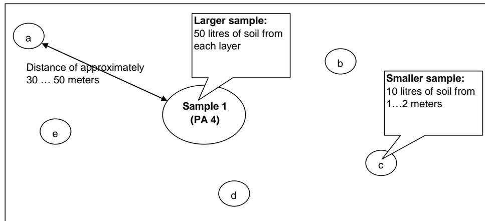
The idea of smaller samples is hereby to study the area conditions in where the larger samples are taken in more comprehensive stabilization studies in geotechnical laboratory.
